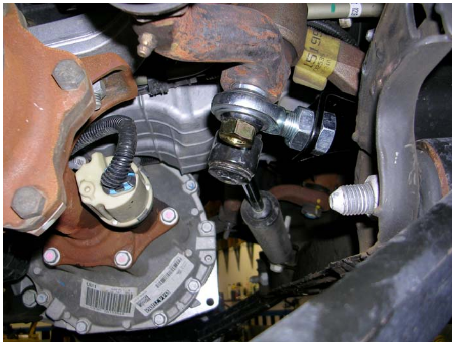
Figure 3: idler arm bracket installed
