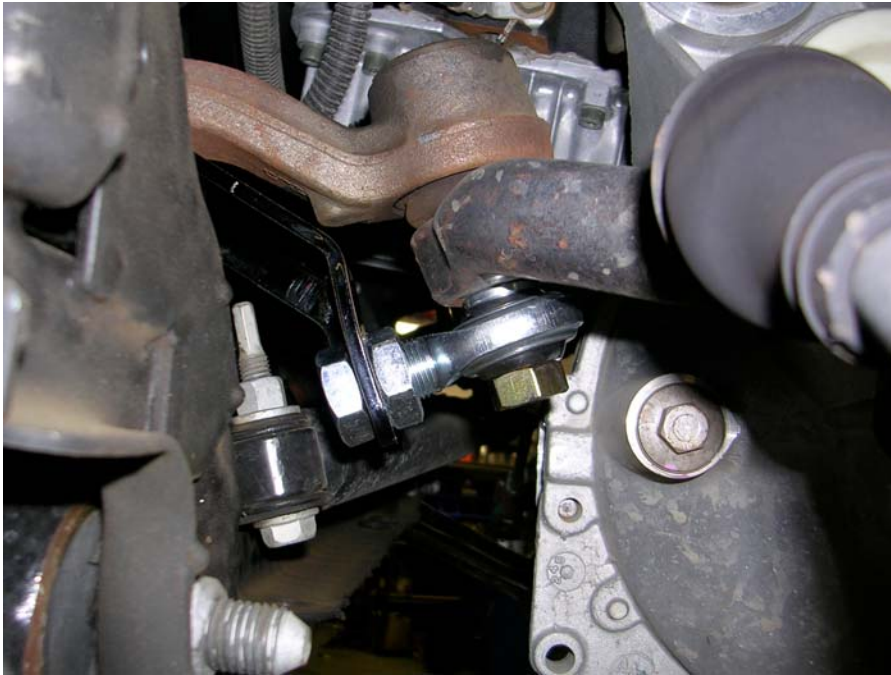
Figure 5: pitman arm bracket installed
